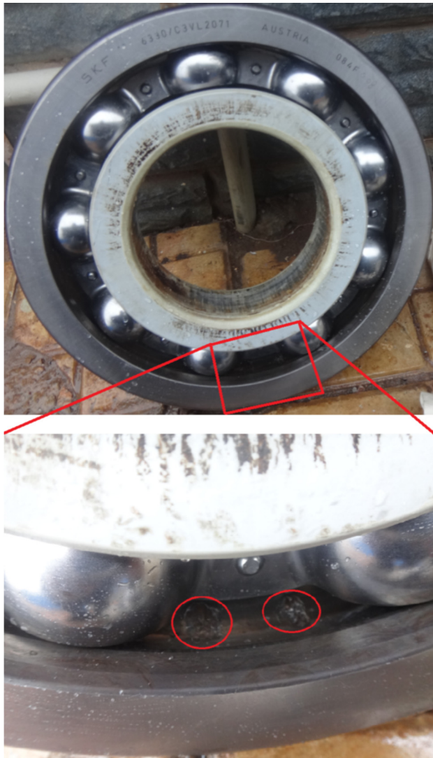
Fig. 7 Disassembled bearing at the drive-end of the generator
